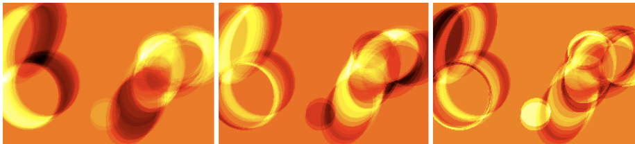
Figure 5: First three eigenimages generated by analyzing the last 20 radar observations, or 10 minutes of real time observations. A maximum of 5 storms was allowed to be active in the environment at any given time. This type of eigenimage provides a good way of extracting short-term motion features based on the past observed radar images.
