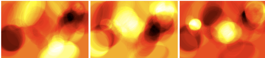
Figure 3: First three eigenimages generated by analyzing the last 100 radar observations. A maximum of 5 storms was allowed to be active in the environment at any given time. Very bright and very dark regions encode places where high variance has been observed, and are related to the direction in which storms are moving.
